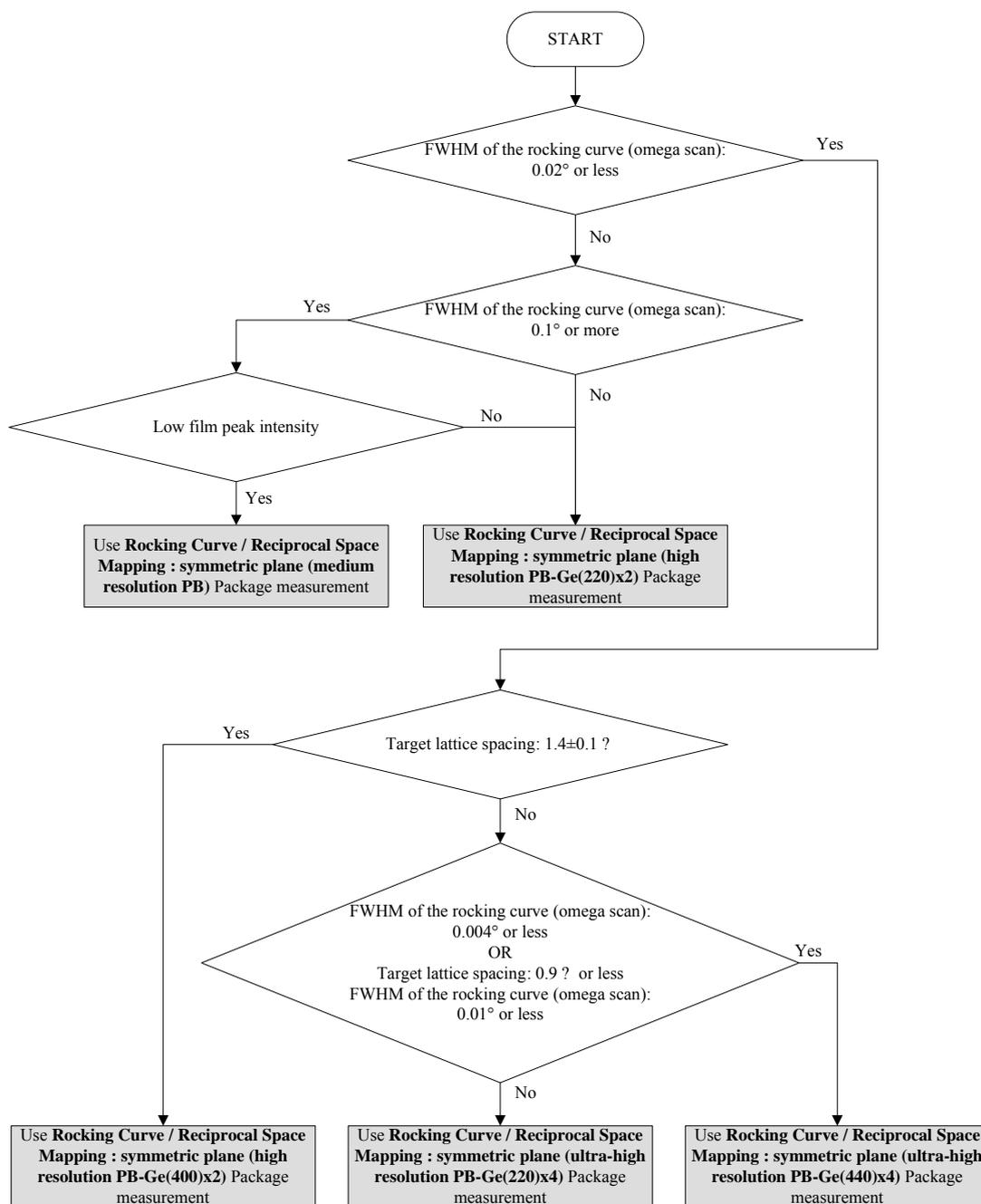
**Fig. 3.1** Selecting a Rocking Curve / Reciprocal Space Mapping Package measurement (incident optics)
