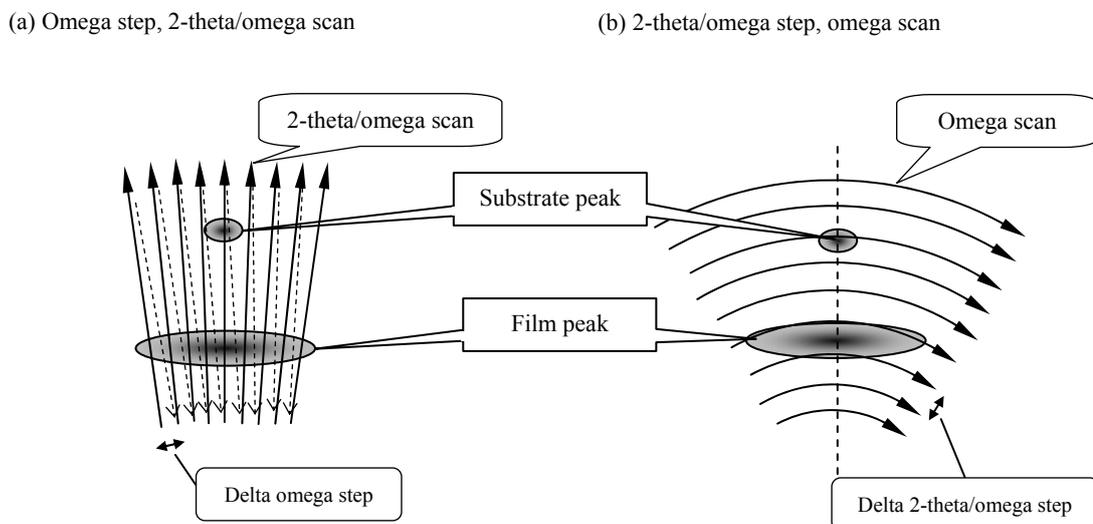
**Fig. 2.3.2 Measurement modes in reciprocal space mapping measurement**
