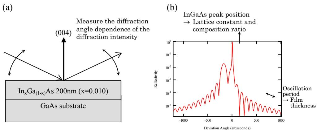
Fig. 2.2.2 What rocking curve measurements of highly crystalline thin film materials can tell us: (a) Measurement diagram
