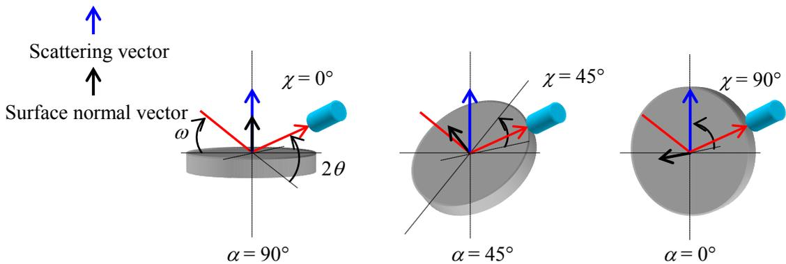
Fig. 2.2.2 Normal pole figure measurement
