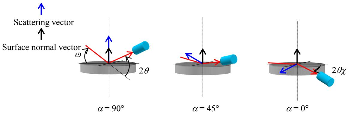
Fig. 2.2.3 In-plane pole figure measurement
