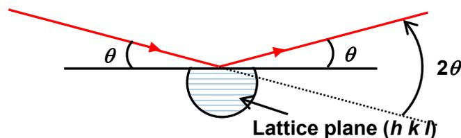
**Fig. 1.2 X-ray diffracted by crystal**
