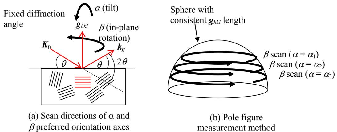
Fig. 2.1.1 Conceptual diagram of pole figure measurement
