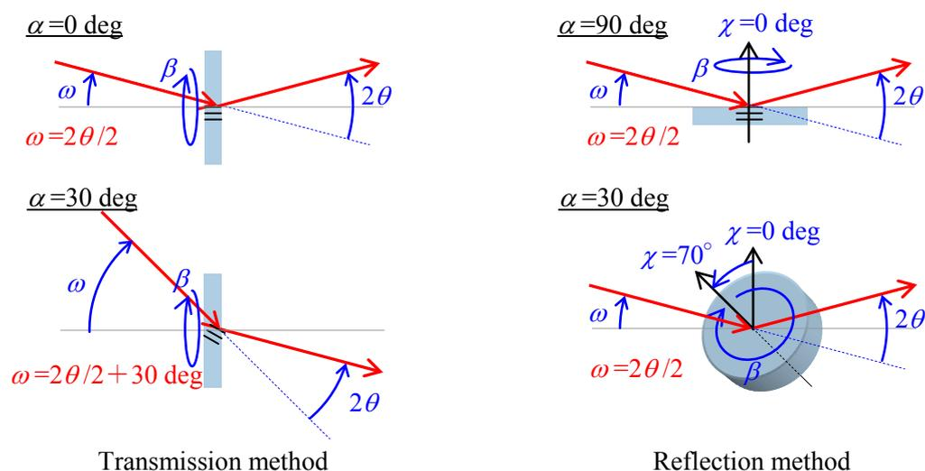
**Fig. 2.2.1 Measurement geometry of pole figure measurement (transmission method and reflection method)**
