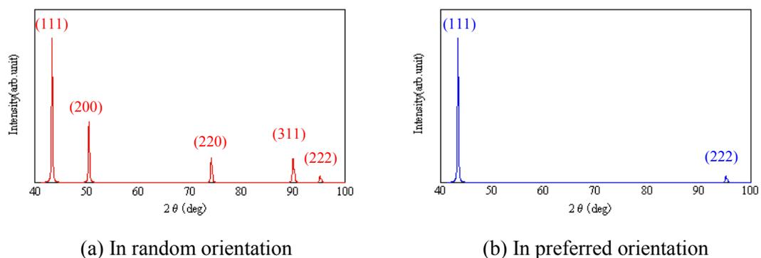
**Fig. 1.3 Patterns of x-rays diffracted by polycrystalline materials**
