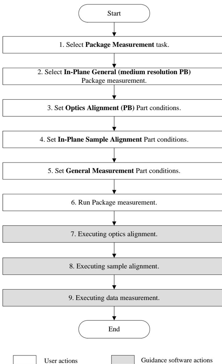
**Fig. 1.1 In-Plane General (medium resolution PB) Package measurement procedural flow**
